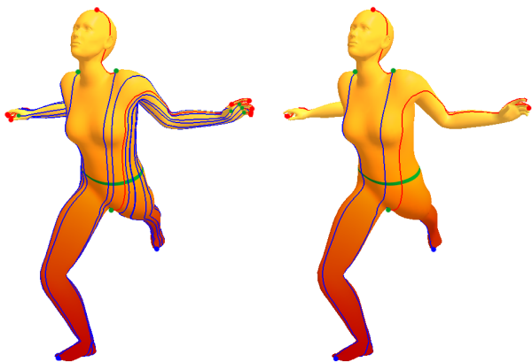
Fig. 7 MS complex of the 1st EF on the dancing lady. Left: full complex, right: simplified complex (only 2 min, 3 max and 3 saddles)
